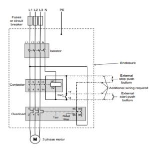
Wiring of additional start stop devices on DOL devices for 240V single phase with 240V coil
