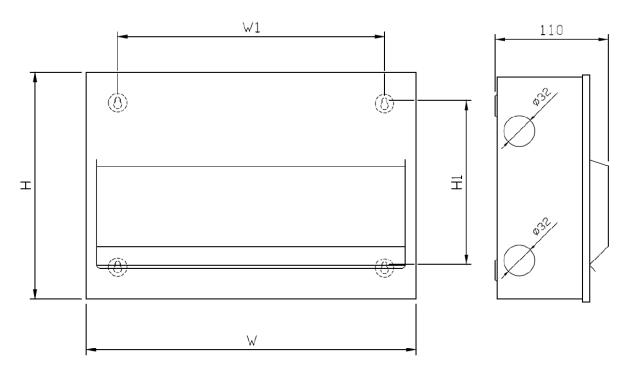
Notes: Knockout placements are symmetrical between top and bottom / left and right sides.
