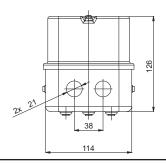
MC18CD for TC1-D Contactors up to 18A
