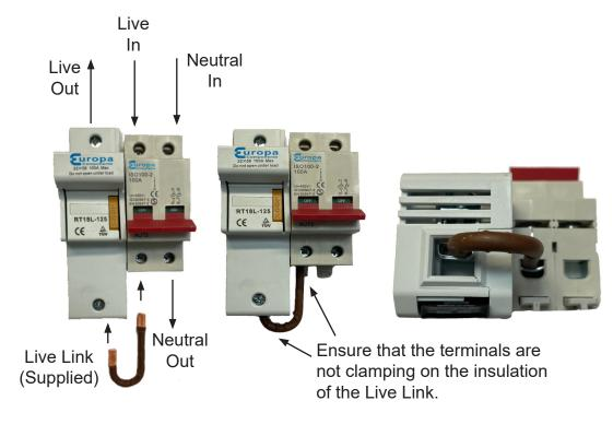
Ensure that the copper link is clamped correctly into the fuse holder and main switch as shown with the recommended torque setting (2.5Nm).
