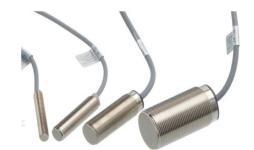
Our inductive sensors are available in M8, M12, M18 and M30. Operating from a 10-30V DC supply and incorporating a "target-sensed" LED indicator, the PNP N/O output stage has a maximum load current of 200mA.
